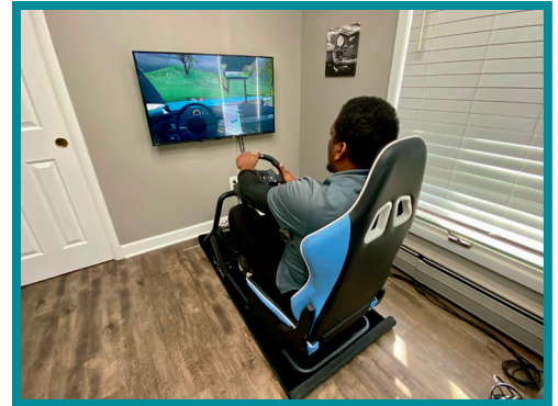
Participants sit in a replicated driver's seat with steering wheel, gearshift, gas and brake pedals, and instrument panel.
